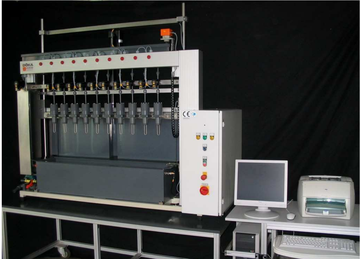
Condom leakage testing device LP-10-C-A (picture shows device with optional accessories)
